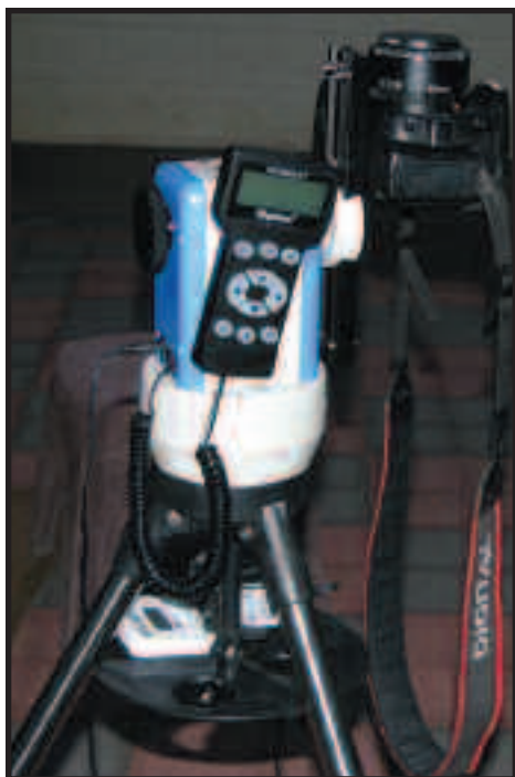
The iOptron Cube is shown with a Canon 20d mounted on the dovetail plate. The mount's accurate tracking permits exposures of up to 60 seconds before field rotation seriously diminishes the results.
