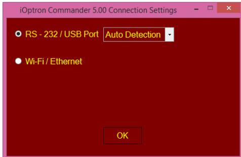
The Device panel will be displayed. Click on the Mount Panel to bring up the Commander for mount setting and direct control. If you are using planetarium software to control the mount, you may just minimize this window.
