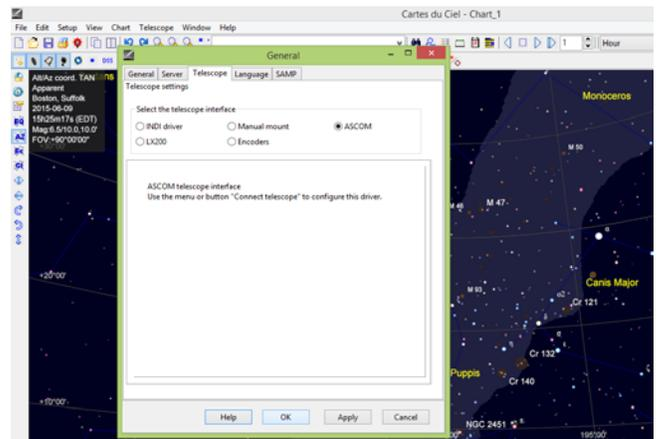
(3) Select **Control panel** in **Telescope** pull-down manual.
