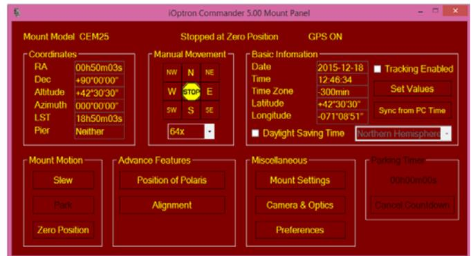
The Commander Mount Panel displays mount model, here is CEM25, with GPS ON but not connected to the satellite and is not slew or tracking. You may click on the related button to perform the mount settings and movements.
