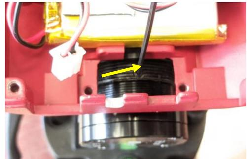
7. Insert optical polar scope into the RA axis. Rotate the front camera mounting adapter to desired orientation and adjust the polar scope so that the LED illuminating hole is facing upward.
