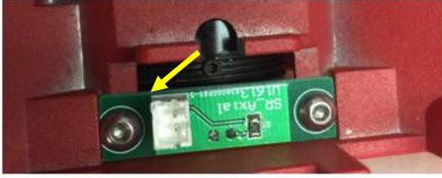
10. Connect the polar scope LED cable between the LED bar and the control board.
