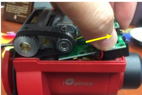
5. Remove polar scope base plate.
