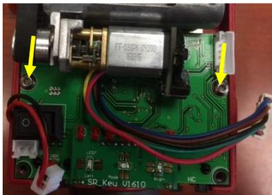
4. Gently pull the circuit board with sockets end up and slide the circuit board out. If the board is stuck by the motor, loosen two Phillips screws hold the motor.
