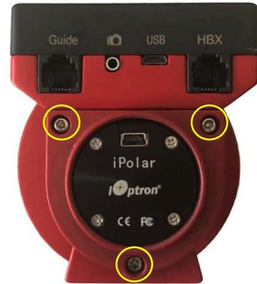
6. Rotate the RA axis to find **TWO** set screws which are used to secure the iPolar in place. Use a 1.5mm hex key to release the set screws. Pull the iPolar out of the RA axle.
