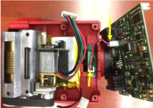
11. Sliding the front end of the control board in. Make sure the LED cable underneath is not jammed.
