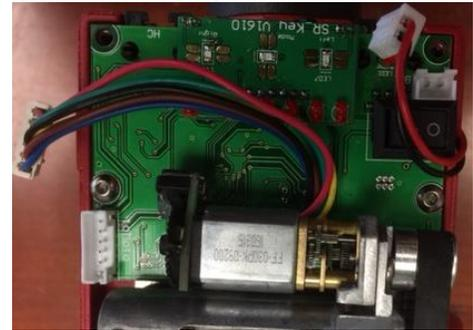
15. Plug in the battery wire and motor cable. Refer to step 2 to wrap the wire properly. Put the cover and screws on.
