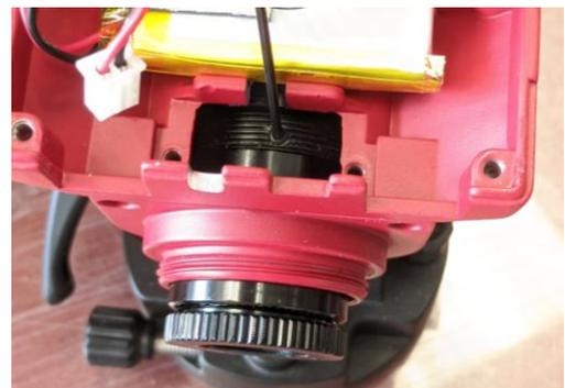
9. Install the polar scope LED abr. Make sure the cable plug is placed on the left side as shown.
