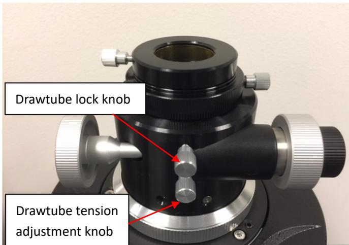
The 8" RC has a 2" linear-bearing Crayford focuser, which has a stabilizing track on the underside of the drawtube that provides extra rigidity for carrying heavy payloads. The tension adjustment knob is on the underside of the focuser while the larger locking knob is on top.
