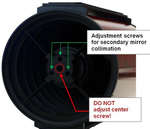
***NOTE: DO NOT adjust the center screw! Only adjust the three screws around the perimeter of the holder! Adjusting the center screw can cause the secondary mirror to fall off and will not be covered under warranty.***
