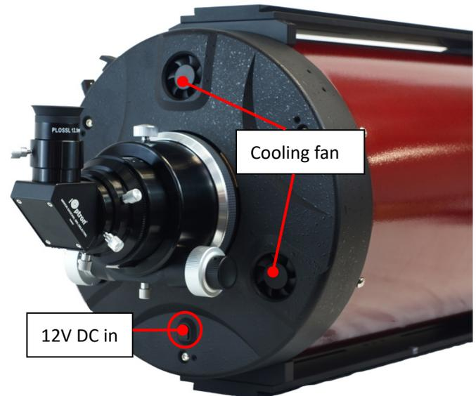
The fans pull outside air in through the rear cell and blow it onto the back of the primary mirror and out the front of the telescope. It's best to point the telescope upward when the fans are on to allow the heat to more efficiently escape. The fans require a 12V power supply; a battery holder using 8 AA batteries is
