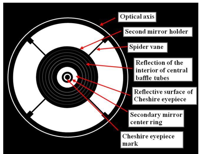
If the scope is in good collimation, the black dot will be dead center in the dark ring, which will in turn be centered in the bright circle. If that's the case, no further adjustments to the secondary mirror will be necessary. The optical axis is denoted by a thin white circle on the outer edge. If this outline is a perfect circle of uniform thickness, no further adjustments to the primary mirror is needed.
