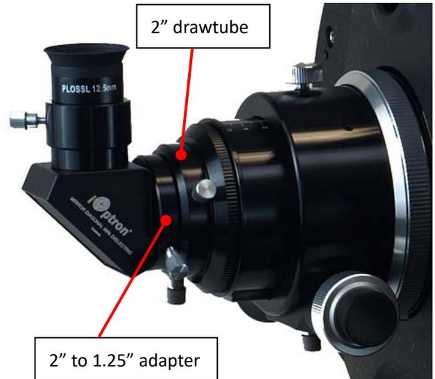
Always begin viewing with the lowest power eyepiece. (Note: a 20 mm focal length eyepiece is lower power than a 10 mm one.) A formula can be used to determine the power of each eyepiece: Telescope focal length divided by eyepiece focal length equals magnification. For example, a RC8 has 1600mm in focal length, the magnification with a 20mm lens is:
