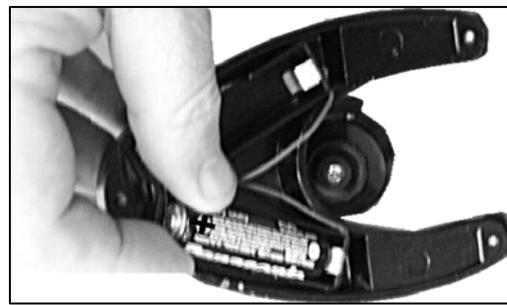
1) You will need to insert two AA alkaline batteries in the base of the microscope. First, you must remove the rubber antiskid bottom cover to access the battery compartment. You will need to use a Phillips-head (+) screwdriver to remove the two screws on this bottom cover. Once the cover is removed, insert the batteries as shown, making sure that the (+) and (-) terminals are properly aligned. Replace the cover and re-insert the screws. Do not overtighten.
