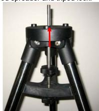
Release three locking screws located at the bottom of the MiniPier body. Put the Base Flange onto the tripod head. Using three M10 hex head screws to secure the base flange.
