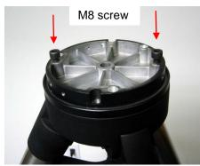
3. Put the MiniPier body onto the Base Flange and secure it using three locking screws.
