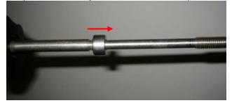
3. Thread the tripod rod all the way up into the threaded hole on the tripod head and tighten it. Lock the tripod using tripod spreader and tripod lock.
