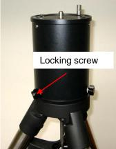
4. Final adjust the tripod height and level the tripod with MiniPier before mounting the iEQ45 mount.
