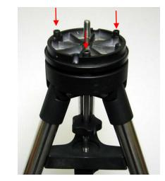
5. Remove the center stud from the top flange by releasing the locking screw from the other side.
