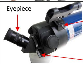
Install the **Finderscope** by sliding the dovetail plate onto the sleeve (see arrow) and tightening the side screw.
