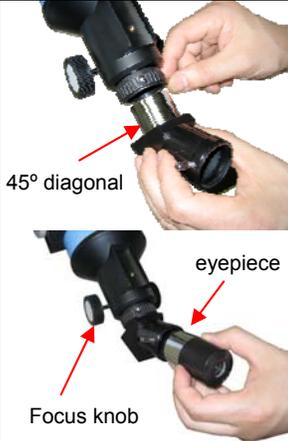
**Insert 45° diagonal:** Insert the diagonal into the eyepiece side of the telescope. Tighten the thumbscrews to a firm feel only.
