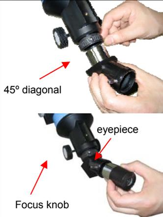
**Insert 45° diagonal:** Insert the diagonal into the eyepiece side of the telescope. Tighten the thumbscrews to a firm feel only.
