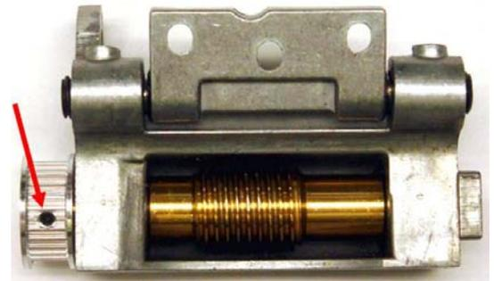
(2) Loosen the two set screws on the old mounting bracket and remove the two brass end caps;
