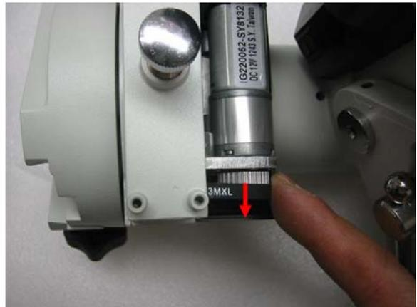
10. Using a 1.5mm hex wrench to loosen the set screw a little on the wheel and remove the wheel from the motor shaft.
