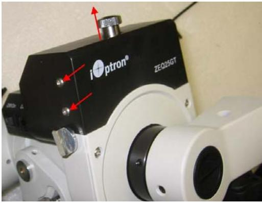
5. Remove R.A. unit cover. If the Guiding port socket prevents a easy pull-off the cover, use a small flat screwdriver to lift the edge a little bit while pull the R.A. cover off, as indicated in the following photo.
