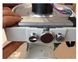
There are two brass washers between the worm assembly and mounting block on the mount.
