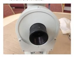
**3.** Remove the both side panels to expose the RA motor and the RA worm assembly.
