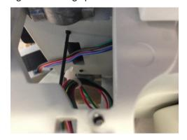
**17.** Insert the RA motor mounting plat from front as indicated in the photo, otherwise it will be difficult to get into the position.
