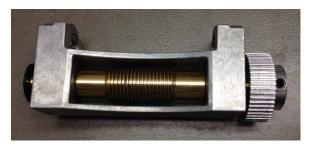
Release one set screw (maybe need to release both of them) and remove the worm end cap. Tap the worm out and replace it. When install the worm end cap, tighten it all the way in then retreat 1/16
