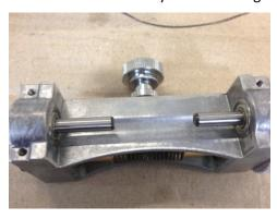
**10.** Remove the pulley and PE encoder index wheel from the RA worm, if it is a non-EC version.
