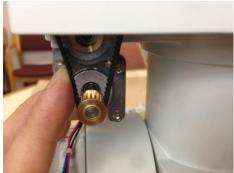
**20.** Check the RS232 and guiding wire bundle to make sure it is not stuck into the space between the RA motor and the mount base. You may pull the wire bundle down.
