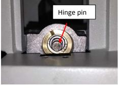
**13.** Tighten the inner positioning end cap, less than half a turn on both sides. Then tighten all the way in. Make sure there is no free play.
