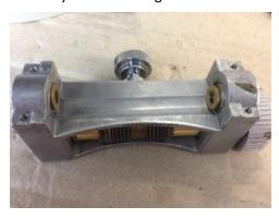
Two hinge pins will be inserted and connected between the holes on worm assembly and mounting block.
