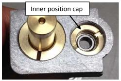
**12.** Insert the worm assembly to the gear box. Make sure that the belt is wrapped onto the pulley. Align the holes and insert one brass washer between them. Insert the hinge pin.
