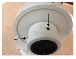
2. Pull the CW shaft mounting house evenly to remove it from the RA axle.
