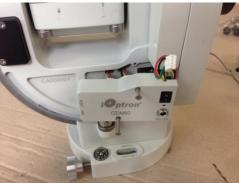
**4.** Remove the RA control board cover to disconnect the motor control cable, if needed.
