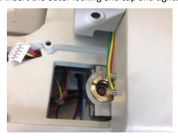
**16.** Tighten the hinge pins set screws.
