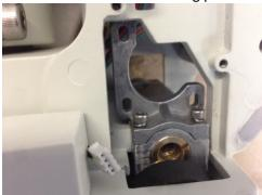
**19.** Adjust the motor position by feeling the belt tension and secure the motor screws.
