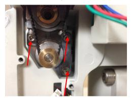
**6.** Remove RA motor mounting plate by remove 4 screws.
