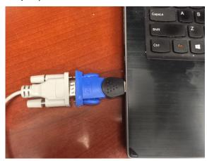
Connect the RJ9 telephone jacket into RS232 port of 8407 HC for hand controller firmware upgrade, or to mount RS232 port (on the base) for mount firmware upgrade.
