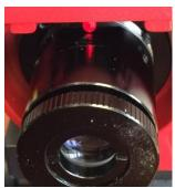
9. Insert the iPolar into the RA axis. Rotate it to align the USB port to the DEC bracket. Lock the set screw gently to secure the iPolar.
