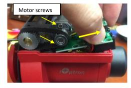
5. Unscrew and remove the polar scope LED board and disconnect wire harness from the main board.
