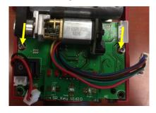
Gently pull the circuit board with sockets end up and slide the circuit board out. If the board is stuck by the motor, loosen two Phillips screws hold the motor.
