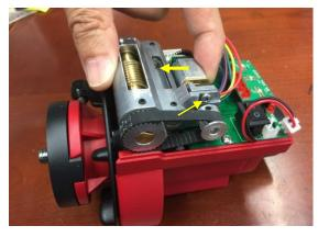
14. When securing the board with two screws, make sure that the battery and wires underneath are properly seated. Fully tighten the screws.
