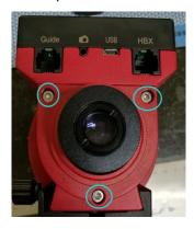
7. Rotate the RA axis to find **TWO** set screws 90 degree apart next to the LED board, which are used to secure the polar scope in place. Use a 1.5mm hex key to release the set screws.
