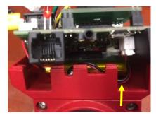
12. Gently push the board in when the power cable goes through the small cut on the board.
