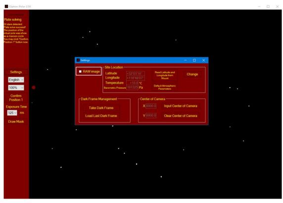
Please check the real time instruction under the **Connected** box on top-left corner. If it displays "xx stars detected. Plate solve succeed!" There is no need to adjust the exposure time. Otherwise, increase the exposure time if it indicates too little stars, or decrease the exposure time when too many stars displayed.
