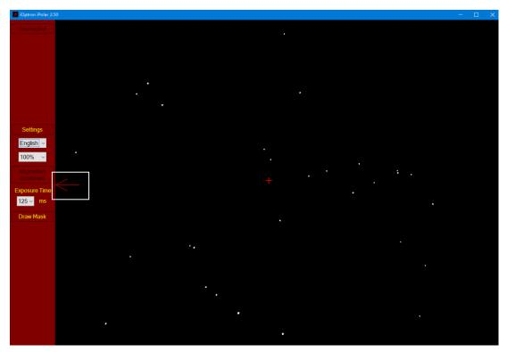
**Camera Center Recalibration**: In the event that the iPolar camera center needs be recalibrated, such as polar alignment result seems not accurate, iPolar was moved, or just want a fresh start, you can go to Settings menu and click on Clear Camera Center button to start over again.
