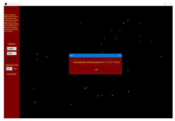
The software will display the virtual pole with a maroon circle and camera center a red cross.
