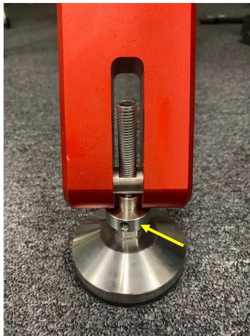
5. To collapse the Tri-Pier 360, loose the Locking Knobs. Pull the collar up while stepping on the Tri-Pier 360 feet.
