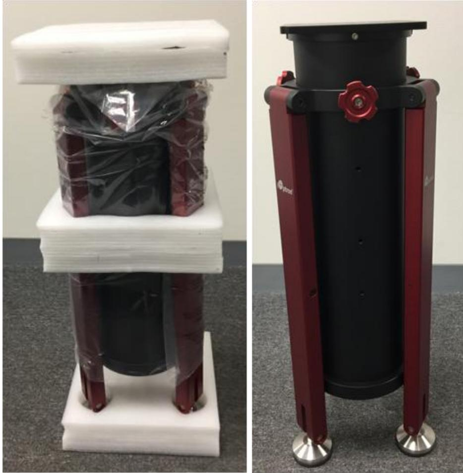
2. Unlock the locking knobs on the mounting collar.
