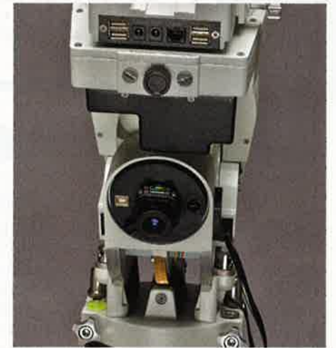
When the view through the included polar alignment scope matches the one "Quick Polar Alignment" shows you, the drive is aligned to our planet's rotational axis.
