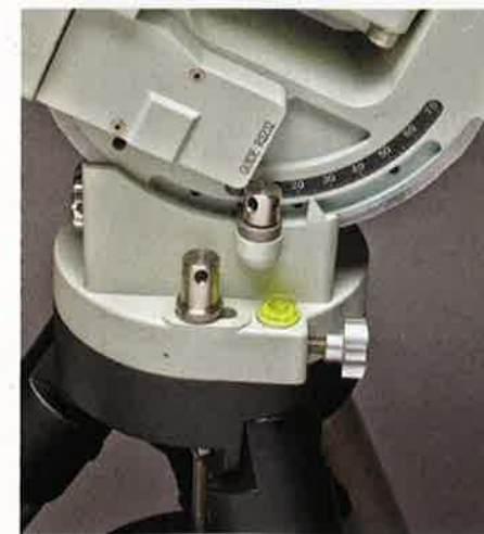
iOptron includes an easy-to-read latitude scale that lets you get pretty close to your northern location. The polar alignment scope then will help you fine-tune this setting.
