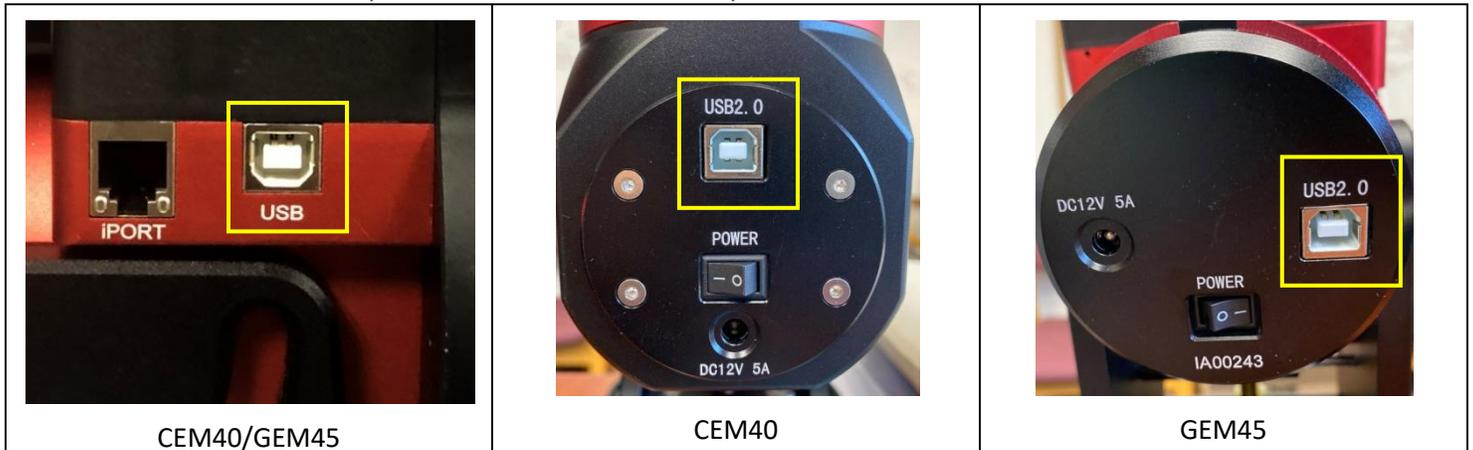
Download FTDI USB to RS232 VCP driver from internet (<https://www.ftdichip.com/Drivers/VCP.htm>), if your computer does not have one installed.
