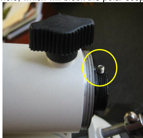
Figure 2. Insert M4 set screw
