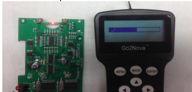
Figure 9. Adjust the LED brightness by a hand controller
