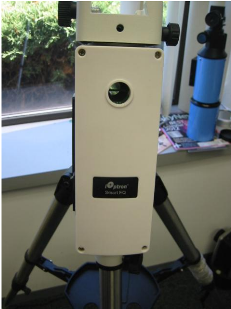
Figure 5. Remove face plate screws
