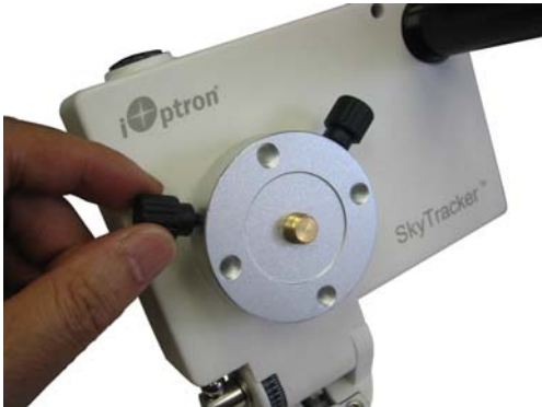
Figure 15. Remove camera mounting block
