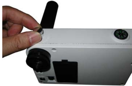
Figure 12. Installed polar scope
