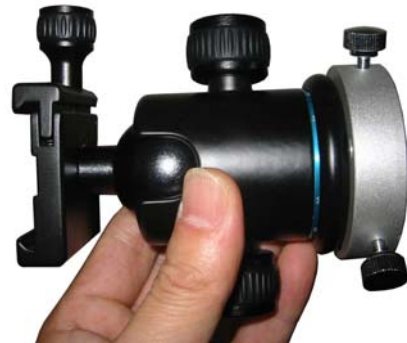
Figure 16. Install ball head
