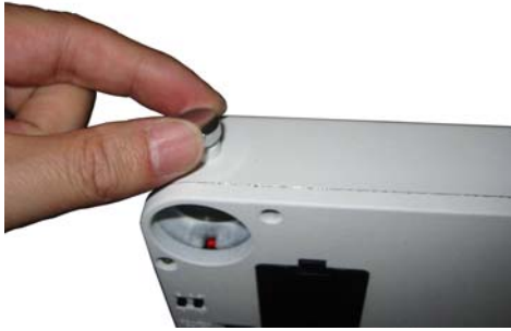
Figure 11. Release polar scope lock screw
