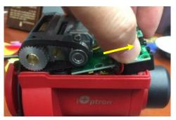
5. Remove polar scope base plate.
