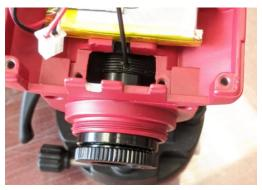
9. Install the polar scope LED abr. Make sure the cable plug is placed on the left side as shown.
