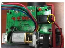
13. If you release the motor to gain more space while remove the board, tighten motor locking screws while push the motor against worm assembly to tension the belt properly.
