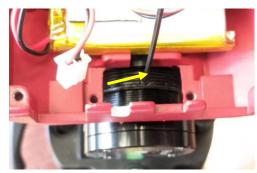
Insert optical polar scope into the RA axis. Rotate the front camera mounting adapter to desired orientation and adjust the polar scope so that the LED illuminating hole is facing upward.
