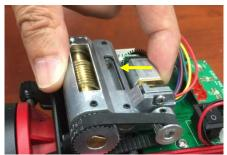
14. When securing the board with two screws, make sure that the battery and wires underneath are properly seated. Fully tighten the screws.
