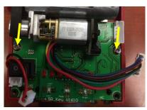
4. Gently pull the circuit board with sockets end up and slide the circuit board out. If the board is stuck by the motor, loosen two Phillips screws hold the motor.
