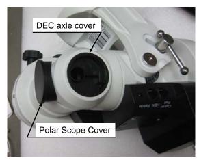
6. Remove a protection tape on polar scope LED Inlet. Insert the polar scope into the scope housing. Make sure 12 o'clock mark is face up (you may use the seam on the DEC body as a reference). Push the polar scope all the way in. The polar scope will be tight fitted into the scope house.
