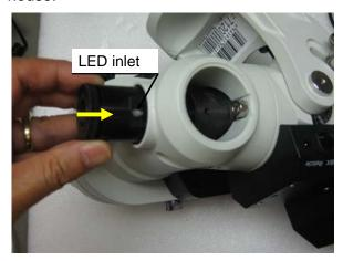
7. Thread in illuminating LED, with a black plastic washer.
