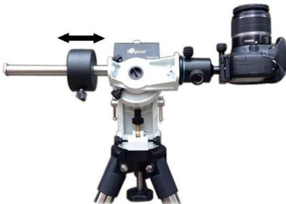
Figure 8. Balance a SkyGuider™ mount
