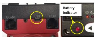
Please don't charge the battery or use USB power when temperature is at or below 0°C (32°F), otherwise the rechargeable battery might be permanently damaged.
