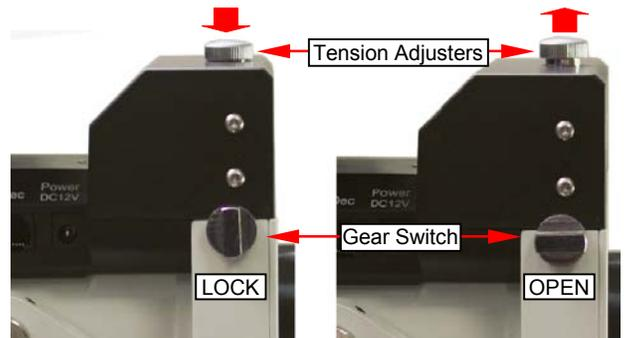
**CAUTION: The balance process MUST be done with Gear Switch at OPEN position! Otherwise it might damage the worm system.**
