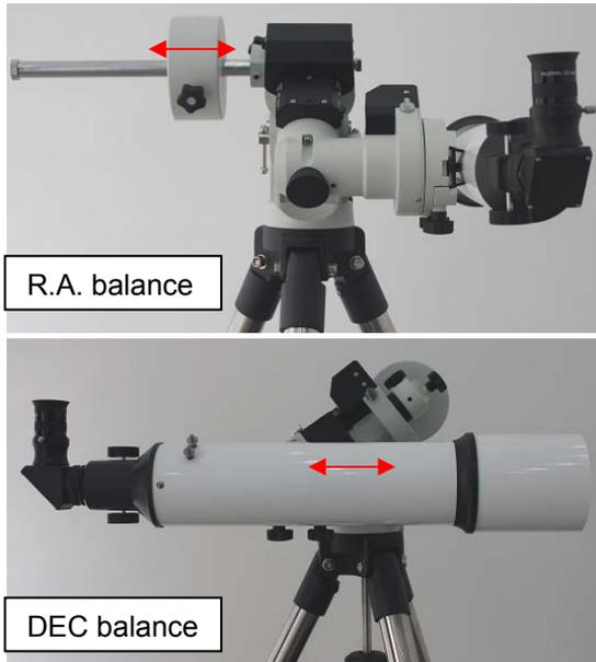
Return the mount to Zero Position after balancing; i.e., CW Shaft points to ground, and telescope tip is at its highest position.
