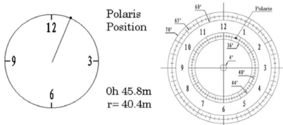
(3) Use the Azimuth and Latitude Adj. Knobs to adjust the mount in both directions and put the Polaris in the location on the Polar Scope Dial (same as indicated on the HC LCD), as shown in the right side of the above figures.
