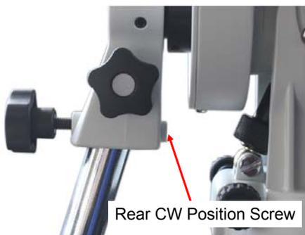
[TIP: At very low latitudes (<math><10^\circ</math>), to avoid CW bumping into tripod leg, turn the Rear CW Position Screw (a hex head set screw) further into CW Mounting Nose before tightening the Front CW Positioning Screw.]
