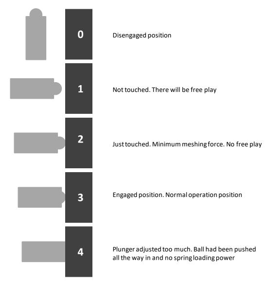
The gear switch should be adjusted to a position that between 2 and 4.
