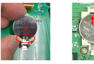
Figure 10. Install a CR2032 battery
