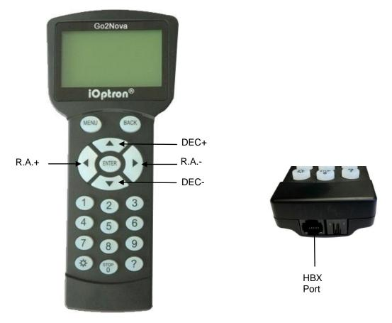
Figure 8. Go2Nova® 8410 hand controller
