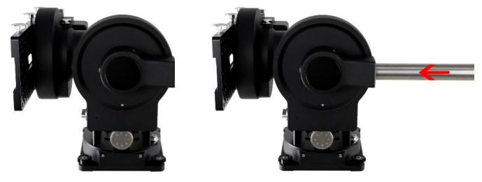
Figure 12. Install CW shaft
