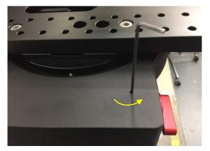
Adjust the **gear adjustment screw** on the side inside 5mm hole by using the 3mm hex key. Turn counterclockwise to loosen the meshing or turn clockwise to tighten the meshing.
