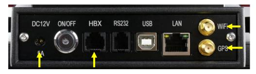
Figure 19. Ports on main control board
