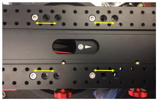
Figure 18. CEM120 dovetail saddle position adjustment
