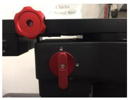
Rotate DEC saddle to exposure two small holes next to DEC **Gear Switch**: one on the top cover (3mm diameter), one on the side (5mm). There is a **set screw** inside the 3mm hole to lock the **gear adjustment screw**, which is inside the 5mm hole.
