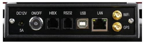
Figure 2. Ports on a CEM120 mount base
