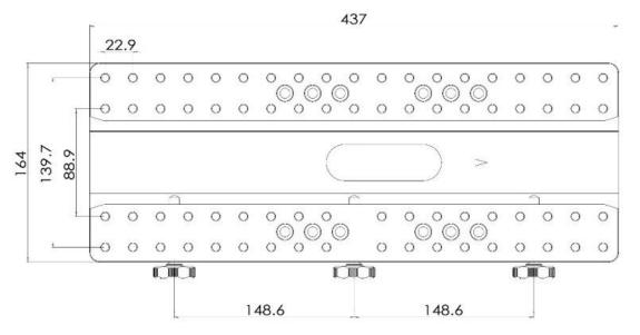
Figure 17. CEM120 dovetail saddle plate
