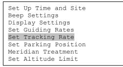
The mount will determine the tracking rate automatically. The tracking rate can be adjusted manually using "**Customer Rate**". The adjustment range is from 0.9900X to 1.0100X of sidereal.
