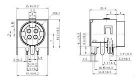
Figure 5. AUX port DIN-422 socket
