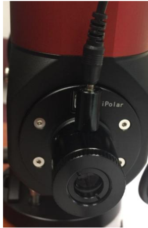
Figure 26. Connect polar scope LED
