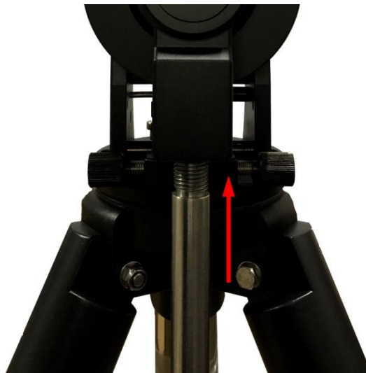
Figure 18. Install CW shaft
