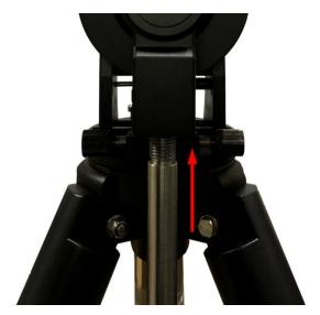
make sure the mount is at its zero position, i.e., CW shaft points to the ground. Disengage the R.A. Gear Switch to set the R.A. axis free before loading the CW. Remove the CW Safety Cap at the end of CW Shaft. Glide the CW over the shaft with the larger hole opening facing down. Tighten the CW Locking Screw to hold the CW in place. Place the Safety Cap back onto the shaft. Move the CW to the bottom of the shaft and tighten the CW locking Screw.
