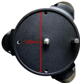
**Set up Mount Head:** Retract the 2x Azimuth (Azi) Adjustment Screws from both sides to leave ample space for the alignment peg to fit in between the 2 Azi Adjustment Screws. Remove the 2x Azi Locking Screws, with washers, from the mount base. Secure the mount head by tightening the Azi Locking Screws
