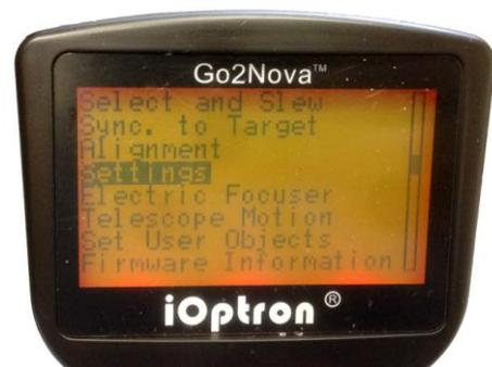
Before GPS picks up signals (before displaying GPS OK), check for **Daylight Saving Time** using arrow key to toggle between **Y** and **N**. Enter the time zone offset to the UTC; for examples:
