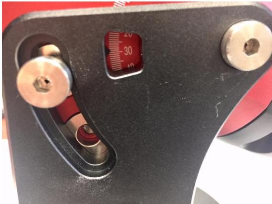
Unthread and remove the Position Bolt to its new location. Adjust the Latitude Adjustment Knob while holding the brass eyebolt until it lines up with the Position Bolt. Secure the Latitude Position Bolt.
