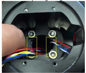
Arrange the wires side-by-side and use a scotch tape to tape them onto the side.
