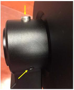
4. Release two set screws on iPolar CEM40 adapter that secure the iPolar inside the RA axle.
