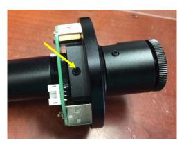
10. There is a fitting opening inside the CEM40 RA axle, with two cutouts on the side for wires passing through.
