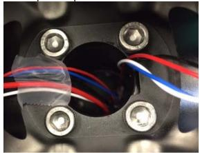
11. Gently insert the polar scope into the RA axle. Secure the CMS cover plate.
