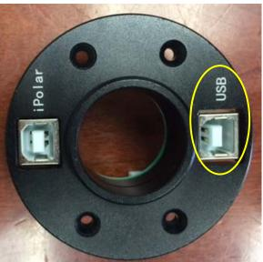
Insert the polar scope into the CMS board, with flat LED window aligned to the iPolar USB port, so the 12 o'clock on polar scope dial will be facing up. Lock the polar scope set screw.
