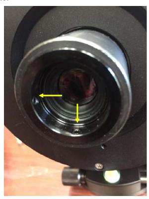
5. Pull the iPolar with adapter and cable out of the RA axle.
