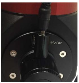
13. Connect the LED cable between the LED and DC 12V output from the DEC saddle.
