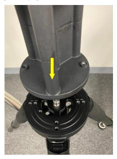
Step 2: Tighten two M6 screws to secure the minipier onto the tripod.
