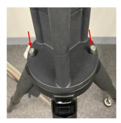
Step 3: Thread the alignment peg on top of the minipier.
