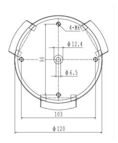
Step 1: Attach the MiniPier onto a tripod, with two holes on the bottom aligned to the threaded holes separated by 103mm, where a mount was secured by AZI locking screws. There is a hole on the minipier base for the alignment peg. You can leave it on the tripod top.
