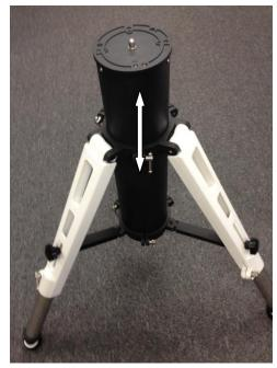
8. Adjust the Tri-pier legs by spreading the legs. Make sure that the Tri-pier feet are sit inside the vibration suspension pads. The pads and the ground surface are contacted well. Tighten the Leg Adjustment & Leveling Screws to secure the Tri-pier.
