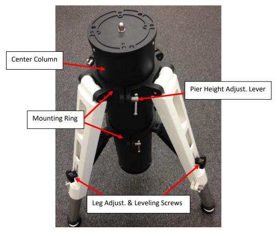
6. There are 6 sets of holes on the Center Column for height adjustment. There are 3 spring balls inside each Mounting Ring to lock the position.
