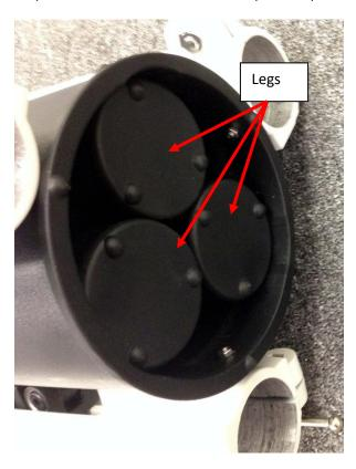
4. Install the leg onto the Tri-pier leg house. Make sure the feet locking screw is aligned to the Leg Adjustment & Leveling Screw.
