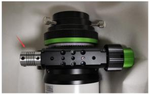
Current, the adapter supports a shaft with a diameter 5, 6, 7 or 8mm. 4mm adapter is optional.
