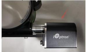
Plug USB cable into the USB port on the iEAF. Connect the other end to a PC for computer control via ASCOM, or plug into a 5V USB charger/power tank to power the iEAF for manual adjusting.
