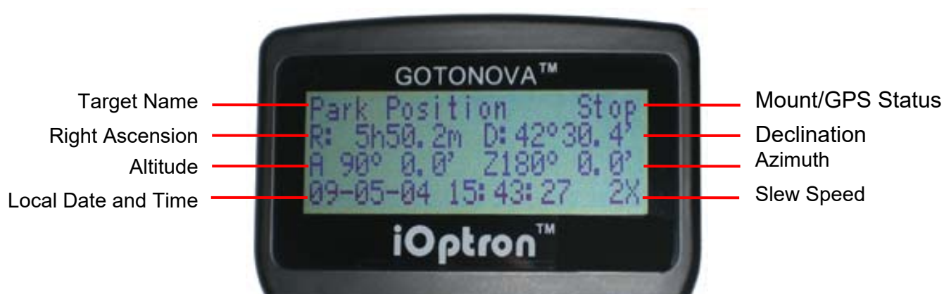
Figure 3. 8405 Hand Controller LCD Information Screen
