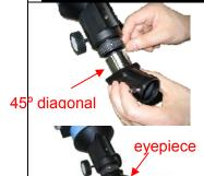
**Insert 45º diagonal:** Insert the diagonal into the eyepiece side of the telescope. Tighten the thumbscrews to a firm feel only.
