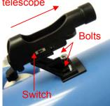
Attach the red dot finder scope to the telescope tube (#1):
