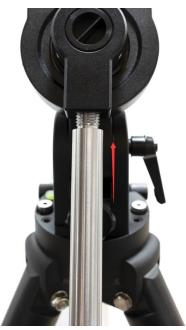
6. <u>Install counterweight</u>: Before putting on CW, make sure the mount is at its zero position, *i.e.*, CW shaft points to the ground. Insert Allen wrench to lock the RA axle and disengage the R.A. Gear Switch to set the R.A. axis free before loading the CW. Remove the CW Safety Cap at the end of CW Shaft. Glide the CW over the shaft with the larger opening facing down.
