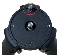
3. <u>Attach mount head</u>: Before put the mount onto the tripod, make sure the RA gear switch is at lock position to prevent mount head free swing by accident! Retract the 2x Azimuth (Azi) Adjustment
