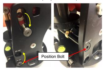
Loosen the Latitude Locking Screws just enough to adjust the latitude setting to 30°. Move the Latitude Locking Screws with washers (one on each side) to the new locations revealed, do not tighten them just yet.
