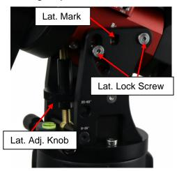
Two latitude ranges, 0~35° and 25~60°, can be set up for the mount head. To change the latitude range from one to the other, **both** the Latitude Position Bolt and the Latitude Locking Screws need to be moved to the correct locations (see photos below).
