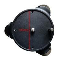
3. Attach Mount Head: Retract the 2x Azimuth (Azi) Adjustment Screws from both sides to leave ample space for the alignment peg to fit in between the 2 Azi Adjustment Screws. Remove the 2x Azi Locking Screws, with washers, from the mount base. Secure the mount head by tightening the Azi Locking Screws into the M6 holes on the tripod. An Allen wrench is included for convenience.
