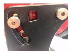
Unthread and remove the Position Bolt to its new location. Adjust the Latitude Adjustment Knob while
