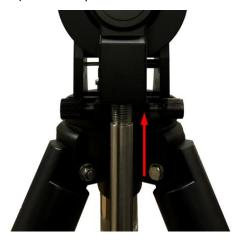
6. Install Counterweight(s): Before putting on CW, make sure the mount is at its zero position, i.e., CW shaft points to the ground. Disengage the R.A. Gear Switch to set the R.A. axis free before loading the CW. Remove the CW Safety Cap at the end of CW Shaft. Glide the CW over the shaft with the larger hole opening facing down. Tighten the CW Locking Screw to hold the CW in place. Place the Safety Cap back onto the shaft. Move the CW to the bottom of the shaft and tighten the CW locking Screw.
