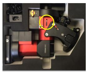
If there is no locking wrench, turn the Gear Switch 90° to lock the R.A. gear system before removing it from the box.
