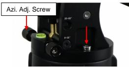
Level the mount by adjusting the tripod legs. Use the build-in Bubble Level Indicator or an external leveler for this purpose.
