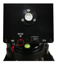
GOTO reference. Without setting the mount zero position properly, it may cause large GOTO error or even cause the scope to hit the tripod leg. The simplest way to find the mount Zero Position of the EQ mode is using the zero position sensors. Press MENU=>Zero Position =>Search Zero Position, then press ENTER. Follow the online instruction to complete process.
