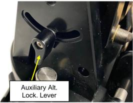
Use the Altitude Adjustment Knob to move the mount to the desired latitude by aligning the scale to the Latitude Mark Line. Tighten both Alt. Locking Knob and Auxiliary Locking Lever. Here the mount is set at 40°. Tighten the Latitude Locking Knob.
