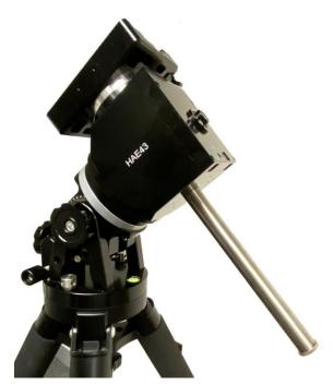
7. <u>Connect cables</u>: Connect the Go2Nova<sup>®</sup> 8409 Hand Controller to the **HBX** port on the mount back. Plug in a 12V DC power supply to the **DC12V IN** socket.
