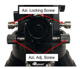
Remove Azi Locking Screws from the mount altitude arm. Secure the mount head by tightening the Azi Locking Screws into the M6 holes on the tripod. There is an Allen wrench stored on the mount base for tightening the screws.
