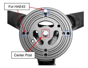
3. Attach mount head: Retract the 2x Azimuth (Azi) Adjustment Screws from both sides to leave ample space for the alignment peg to be fitted in between the 2x Azi Adjustment Screws.
