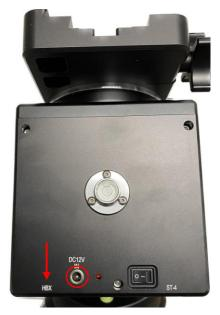
7. <u>Set Zero Position</u>: The Zero Position is the mount GOTO reference. Without setting the mount zero position properly, it may cause a large GOTO error or even cause the scope to hit the tripod leg. The simplest way to find the mount Zero Position of the EQ mode is using the zero position sensors. Press MENU=>Zero Position =>Search Zero Position, then press ENTER. Follow the online instruction to complete the process.
