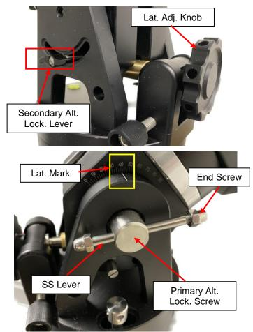
Use the Latitude Adjustment Knob to move the mount to the desired latitude by aligning the scale to the latitude Mark Line. Tighten both Primary Locking Screw and Secondary Lever.
