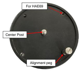
**3.** <u>Attach mount head</u>: Retract the 2x Azimuth (Azi) Adjustment Screws from both sides to leave ample space for the alignment peg to be fitted in between the 2xAzi Adjustment Screws.
