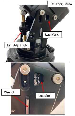
Insert the Allen wrench into the Latitude Adjustment Knob for more turning torque.
