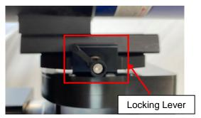
Pull the lever and turn it to the position that the lever is parallel to the saddle or points towards the scope to prevent it interfering with the DEC unit during mount GOTO and tracking.
