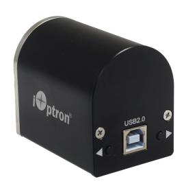
The new iOptron Electronic Automatic Focuser (iEAF) is designed for both Crayford and Rack-and-Pinion focusers. It is powered by a 5V USB port. The focuser is ASCOM compatible and will work with most planetarium and imaging software. It also can be adjusted manually by pressing the buttons on the focuser.
