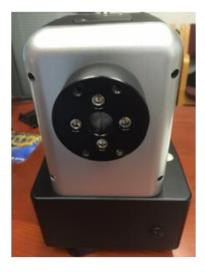
10. Attach the dovetail saddle and make sure that the arrow is pointing upward.
