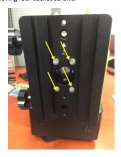
6. Further remove the dovetail mounting ring.
