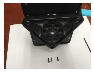
Remove two hex head screws with a 2mm Allen wrench.
