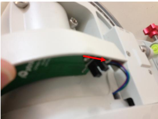
Slightly separate the RA board case from the RA worm wheel case. Unplug the motor control cable.
