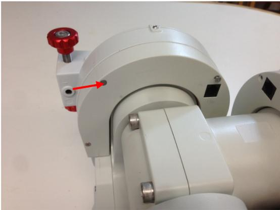
Rotate the mount head to sideway. Remove four screws that hold the RA board cover.
