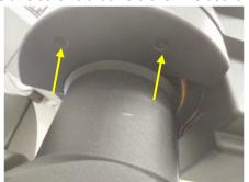
3. Remove two screws under DEC ring gear compartment.
