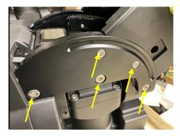
4. The motor was secure by 3 socket screws. To adjust the belt tension, loosen these screws a little bit.
