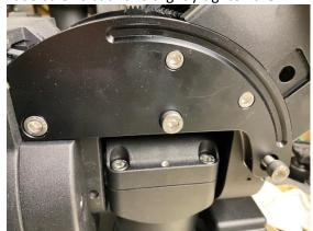
9. Remove two screws that hold the RA control board cover to expose the cables that go to the RA board.
