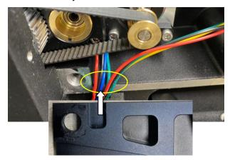
13. Slide the side panel on and arrange the cables to go into the slot.
