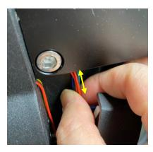
16. After secure the side cover. Put the altitude locking screws back and lock it.
