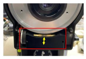
4. If the RA worm assembly is moving left and right with turning the RA axle gently, it means there is a small gap between the RA worm assembly and mounting house. It can be eliminated by tightening the bearing end caps. **Refer to Step 6 for how to fix.**
