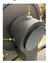
2. Remove RA ring gear cover to expose the ring gear and worm assembly. Remove RA axle locking Allen wrench and engage the RA gear switch.
