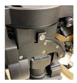
7. Release altitude locking screws on both sides. Turn the altitude knob to adjust it to ~ 40 degree to expose the RA motor and belt. Lock the GPS side altitude locking screw but remove motor side one.
