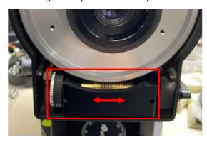
5. If the brass RA worm, or the worm pulley is moving left and right with turning the RA axle gently, there is a gap between the RA worm and worm bearing. It can only be fixed by removing the RA worm assembly and tightening the RA worm end cap.
