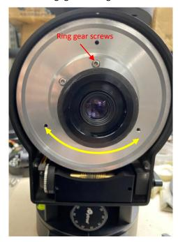
Check six (6) Ring gear screws to make sure they are tightened properly. Gently turn the ring gear and check the worm and worm assembly movement.
