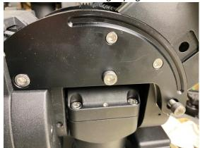
15. Remove two screws that hold the RA control board cover to expose the cables that go to the RA board. And slightly pull the cables to make sure they move freely.
