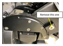
8. Remove 5 socket screws to separate mount left base supporting plate.
