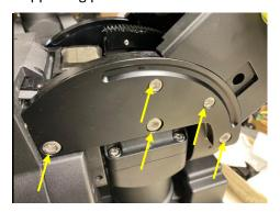
The worm assembly is attached to the mount via to hinge pins via bearings. There are two set screws to fix the pins in place. There is an brass end cap to secure he bearings and asset screw to fix the end cap.
