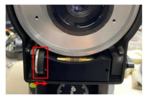
Set the mount to Zero Position. Locking RA axle by insert the locking Allen wrench. Release RA gear switch but keep the DEC gear switch engaged. Flip the mount head to let it sit on dovetail saddle.
