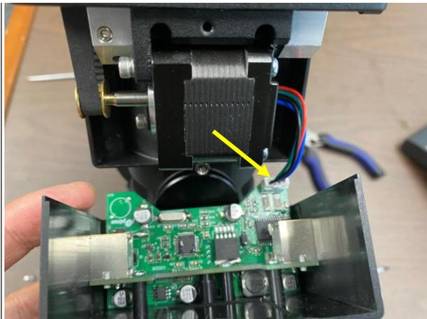
3. Unscrew the screw post to expose the hole on the mount DEC axle housing. You may need a pair of pliers to turning the post.
