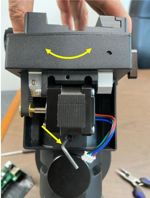
Carefully adjust the wrench position to make sure that it is fully engaged with the set screw. Turn half turn counterclockwise to release the set screw. Do NOT turn too much or you may lose set screw!
