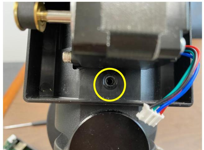
4. The DEC axle is mounted inside the housing with a bearing locking nut. It was tightened using a pair of special nose pliers. Then locked by a set screw, which can be accessed through the screw hole above.
