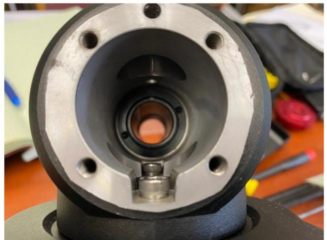
Since we do not have the tools to release the locking nut, we'll use a small wrench to do it.
