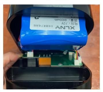
5. Align the cover to the mount body at the bottom first, with screw holes aligned. Push the wire in if it get into the cover and mount frame.
