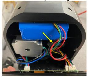
8. Connect the wire and put the cover on.
