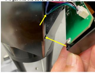
Then align the cover top to the battery and push the battery in with the cover. The cover should sit flush with the mount body.
