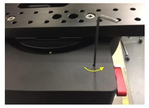
Adjust the **gear adjustment screw** on the side inside 5mm hole by using the 3mm hex key. Turn counterclockwise to loosen the meshing or turn clockwise to tighten the meshing.
