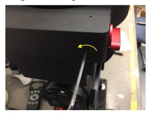
If the motor stalls or the mount does not tracking smoothly, most likely the meshing is too tight. You may loosen it by about 1/8 turn (or less for tracking). *Tighten the set screw to LOCK the gear screw (important)*, then test the mount. Adjust again if needed, but no more than 1/2 turn in total.
