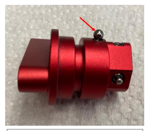
The ball bearing will stay on top of the spring and outside the gear switch hole. The ball will be lost easily during removing or installing the gear switch. To install, the ball bearing and spring need be pushed down into the hole while inserting the gear switch into the mount.
