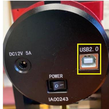
USB port on back of RA axis (CMS input)
