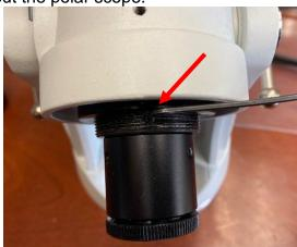
3. Insert the iPolar into the RA axis. Lock the set screw gently to secure the iPolar.
