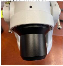
2. Find the polar scope locking screw and use 1.5mm hex key to release it slightly and pull out the polar scope.
