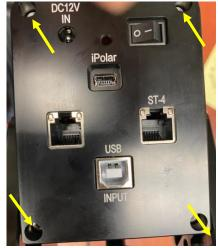
Thread the iPolar cable to the front opening and plug one end into the iPolar port on the main board. Closed the main board cover and secure the screws.
