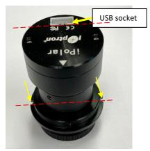
4. Tighten two iPolar setting screws. Do not over tighten them, or the lens tube may be damaged.
