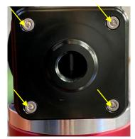
6. Remove four socket screws that hold the control board cover.
