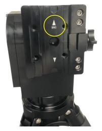
5. Attach telescope: There are two arrows on the dovetail saddle. One is for telescope mounting (dovetail saddle side-mounted) and the other is for binocular (dovetail up-mounted). Slide the telescope/binocular into the dovetail saddle. Make sure that the objective end is pointing to the direction as the arrow mark on the dovetail pointed to.
