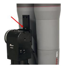
6. <u>Connect cables</u>: Connect the Go2Nova<sup>®</sup> 8409 Hand Controller to the **HBX** port on the mount back. Plug in a 12V DC power supply (5.5/2.1mm plug, center positive) to the **DC12V IN** socket.
